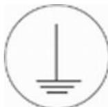
This symbol labels the connection points for the **protective conductor connection**.
