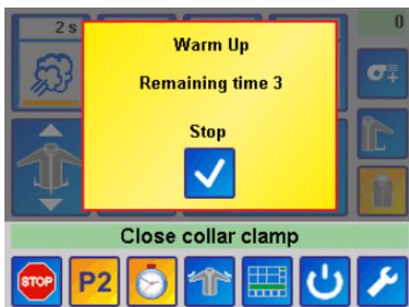
Fig. 72: Stopping energy-saving mode
