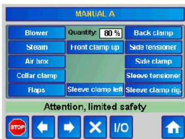
Fig. 20: Manual mode touch screen (EN)
