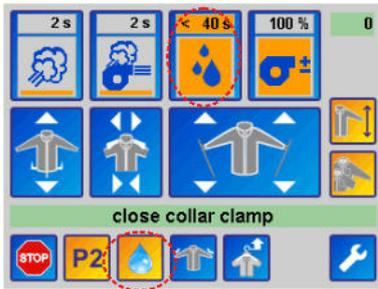
Fig. 67: Residual moisture control screen
